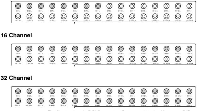
The video inputs are 75  $\Omega$  BNC connectors. Plug one end into the video source (DVD, Camera, etc.) and plug the other end into the desired BNC input on the recorder.
